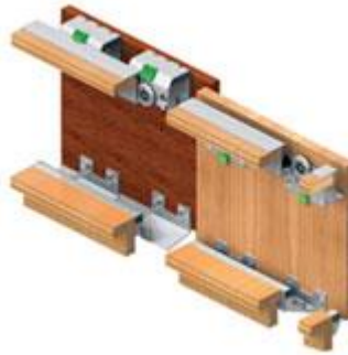
Gm 10-3 Sliding System 50kg Door Thickness two door wardrobe
